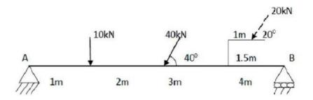
Determine the reactions at supports for the beam.
